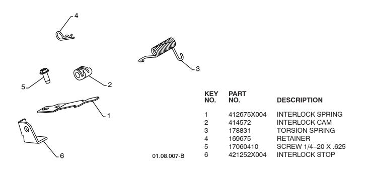
**NOTE:** All component dimensions given in U.S. inches. 1 inch = 25.4 mm **IMPORTANT:** Use only Original Equipment Manufacturer (O.E.M.) replacement parts. Failure to do so could be hazardous, damage your snow thrower and void your warranty.
